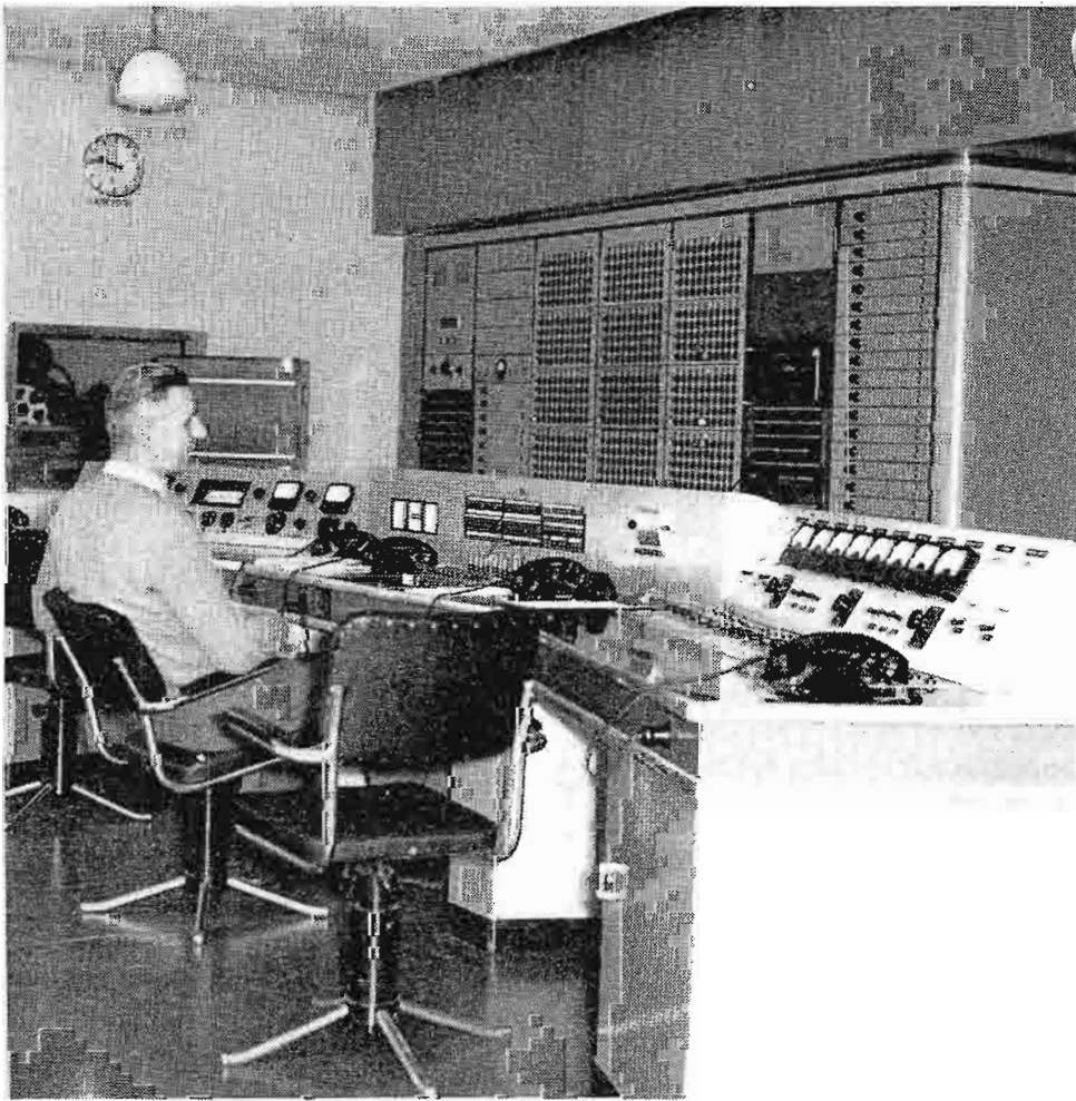
FIG. 10. Master control at Munich Studios feeds program signals to transmitters for target countries. (This unit was designed and built by RFE engineers.)
